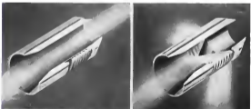
ARTIST'S DRAWING OF REVERSER reverser showing retracted flow and then reverser taking hold. Blocking vanes are retracted into stream for full forward thrust and swing out into stream for reverse thrust.
